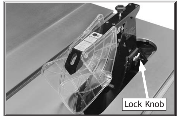
Figure 5. Location to secure blade guard.
